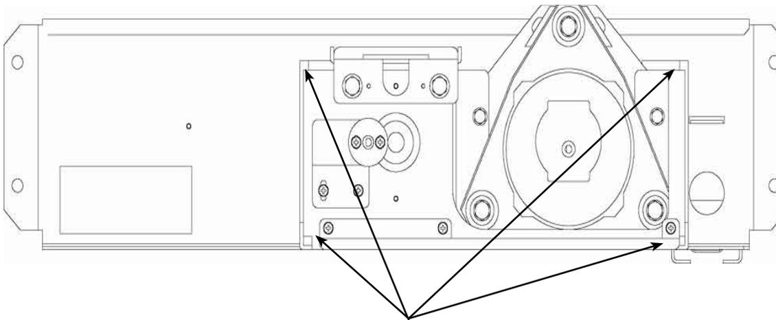
Remove the Hardware from the control panel plate and separate the Steering Handle Assy from the plate.
