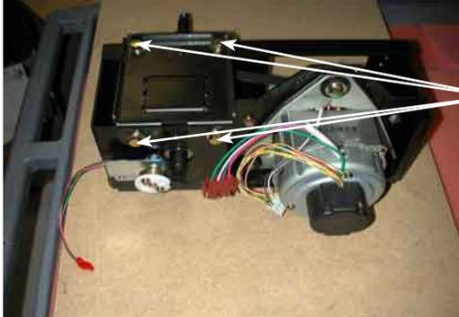
Remove these 4 13mm bolts to remove the stopper plate from the assembly.
