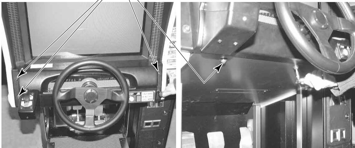
Unplug the 5 connectors and remove the Control Panel. Be careful not to damage any of the wiring.
