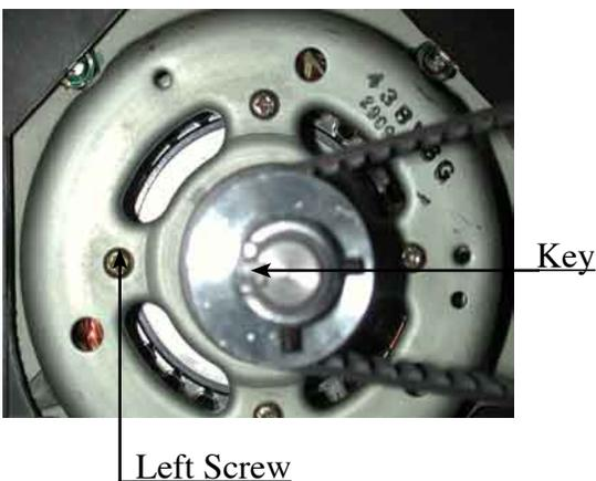
Then turn the motor until the key points to the left screw on the motor.
