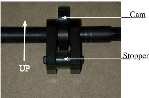
Be sure to center the shaft with the cam in the upwards position and the Stopper dangling downwards.
