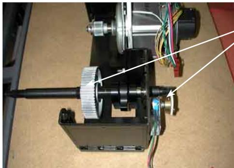
Slide the shaft out of the housing having a care for the volume pot in the rear. Using a 2mm Allen wrench, remove the pulley from the shaft.
