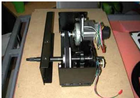
Slide the front plate off the assembly and off the shaft. Then remove the belt from the two pulleys of the motor and the shaft.
