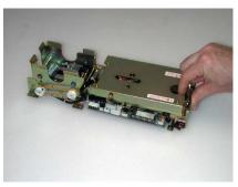
1- Access the transport area by releasing the top door stay mechanism. (Green Bar)
