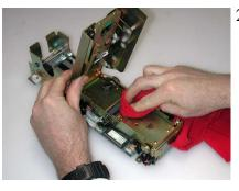
2- Using a red shop rag and denatured alcohol, thoroughly wipe down lower transport area.
